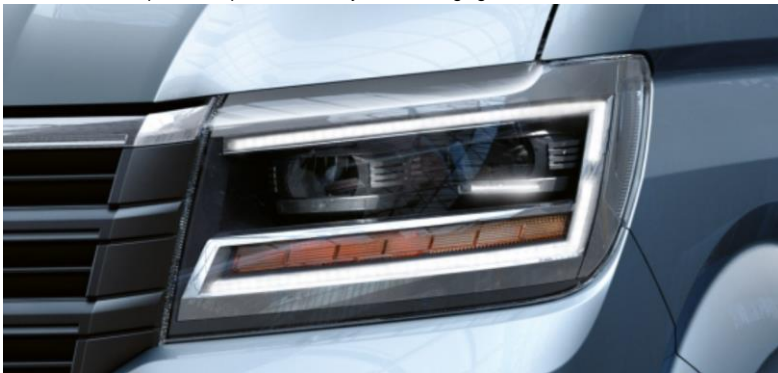
3 – LED headlamps with separate LED daytime running lights
